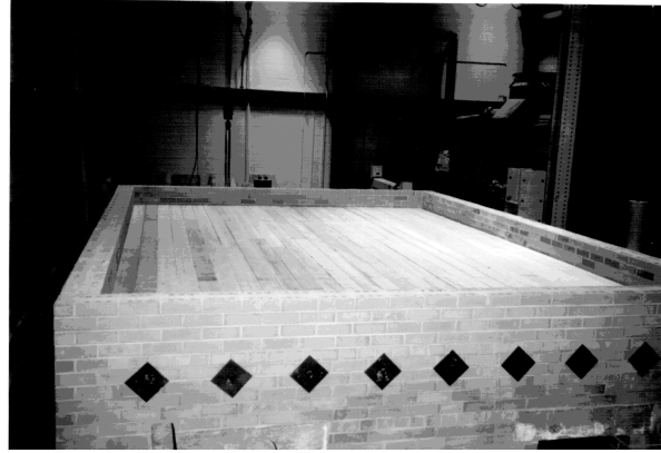
Figure 2: Anchored wood floor
