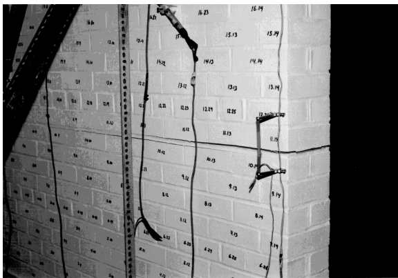
Figure 4: Clip gage recording rocking motion
